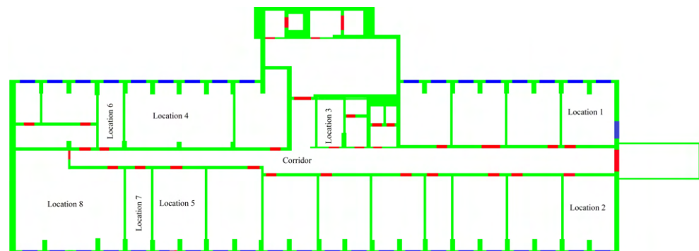
Figure 2. Measurement locations at DIET Department. Green, blue, and red lines represent walls, windows, and doors, respectively.
