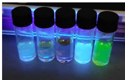
Figure 5.2 Aqueous solutions containing some of the organic salts, under irradiation with a 365 nm lamp; from left to right, PEPyI 2 , TBMPyI 2 , BTBMPyI 2 , MDAPI 2 and MDPPI 2 .
