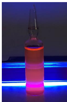
Figure 3.3 Fluorescence of AEPyI 2 in aqueous solution, under excitation with a 365 nm lamp.
