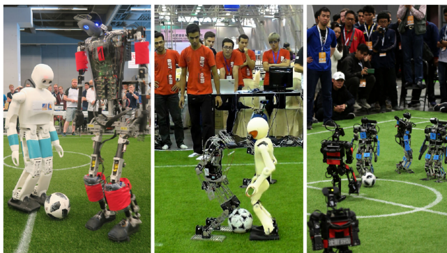
Fig. 5. HLs: HASL, HTSL, and HKSL. The number of robots per team goes from no more than two in the HASL to at most three and four robots in the HTSL and HKSL, respectively. The dimensions of the robots are 130–180 cm in HASL, 80–140 cm in HTSL, and 40–90 cm height in HKSL. The ball used is the FIFA size 1 for HKSL, size 3 for HTSL, and size 5 for HASL. The playing area of the field is 14 \times 9 m in the HASL and 9 \times 6 m in HTSL and HKSL.
