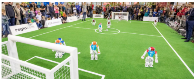
Fig. 4. SPL. The platform is the humanoid NAO robot which is 57.4 cm \times 31 cm \times 27.5 cm in size. In this league, each team is composed by not more than five players. The field size is 9 times 6 m and the ball used is black and white with 100 mm of diameter.
