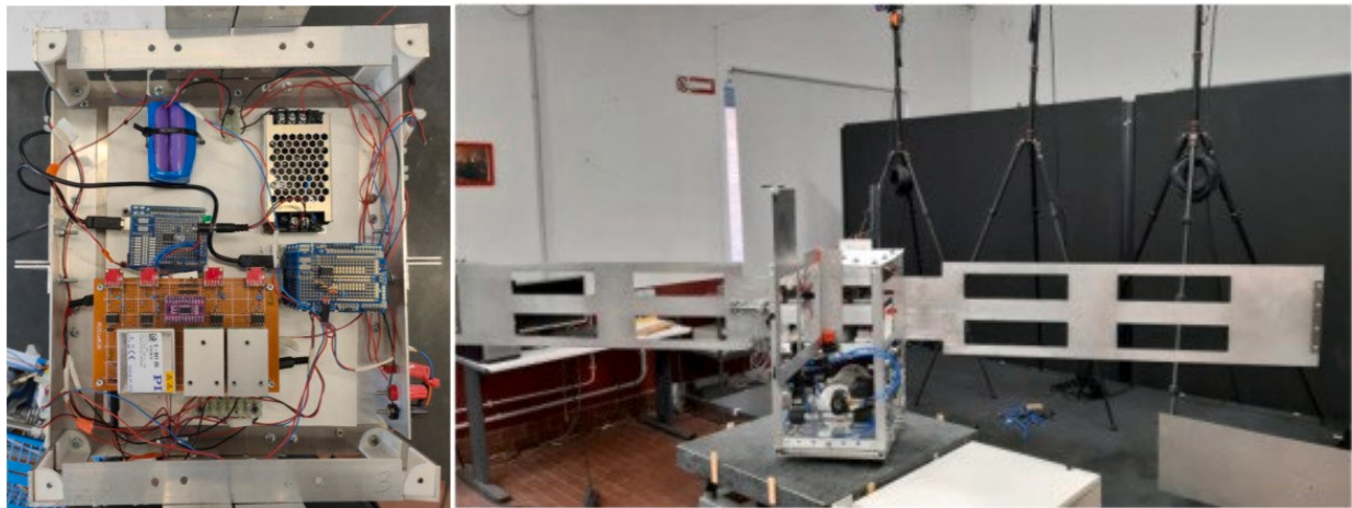
Fig. 3 Electronics compartment (left) used for vibration sensing and control of the highly flexible appendages (right).
