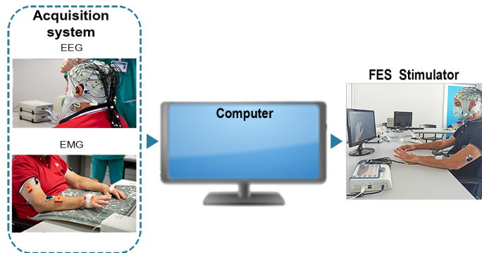
Figure 5.1. The h-BCI components: the acquisition system acquires the EEG and EMG signals through EEG active electrodes and EMG wireless sensors, and sends them to a computer where they are processed in real-time to detect a correct movement and trigger the FES stimulator to deliver the stimulation to the patient.
