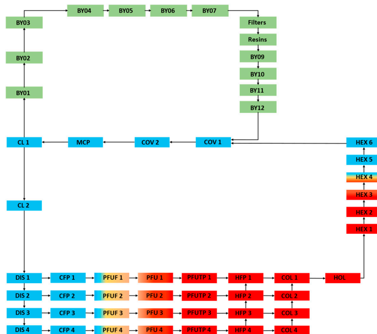
Figure 2. EU-DEMO divertor PFU PHTS OSCAR-Fusion model.
