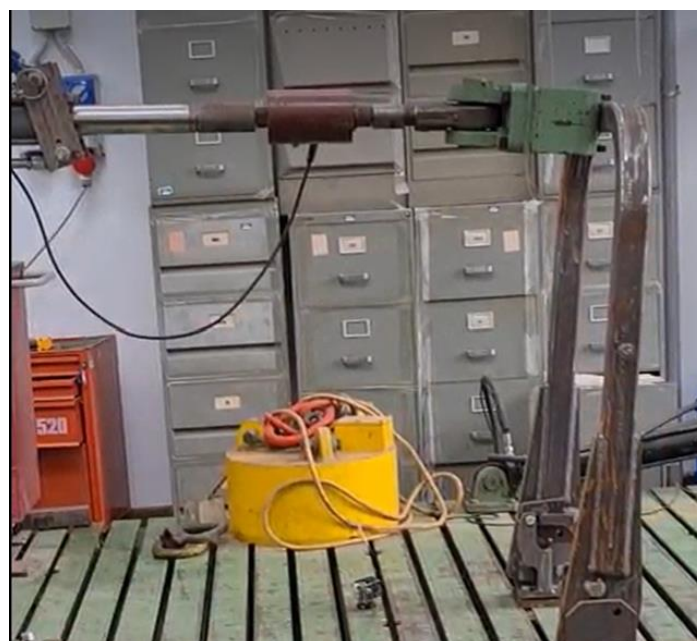
Figure 14. Application of a longitudinal force to test the behavior of the ALD.
