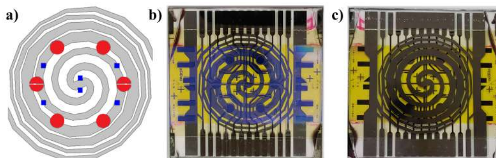
Figure 4. (a) Geometry of the thin film heater (gray lines) overlapped by red circles, that indicate the photosensors, and by blue squares, representing the temperature sensors. (b) SoG top side, hosting photosensors, temperature sensors, and interferential filter (light brown rectangular band). (c) SoG bottom side, hosting the thin film heater.
