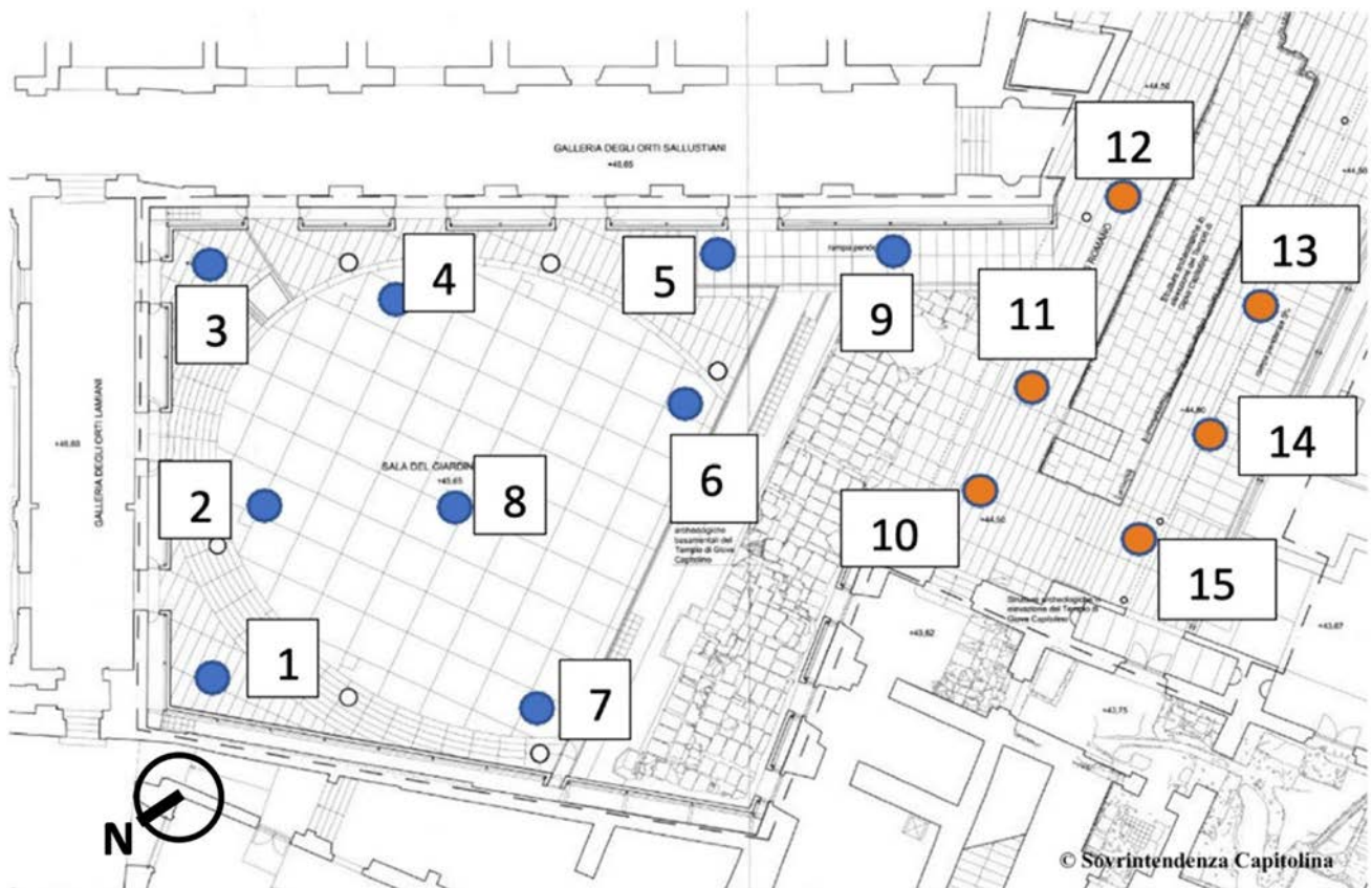
Fig. 12 Position of the laser scanner during data collection process at Sala del Giardino Romano (in blue) and Galleria del Muro Romano (in orange) (color figure online)
