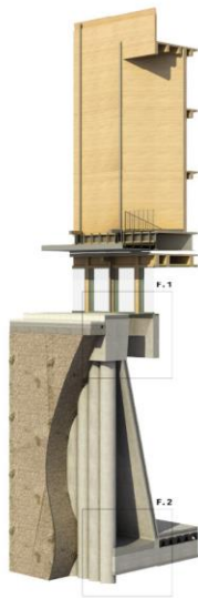
Figure 7. North Side Rendered view. Section of: (i) basement: bulkhead and foundation slab, (ii) upperbuildings: timber-steel columns, isolation and the timber structure.
