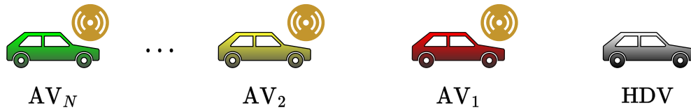
Figure 7.1. AVs platooning system scenario. Each AV is equipped with a range sensor to estimate the space gap from the vehicle ahead.
