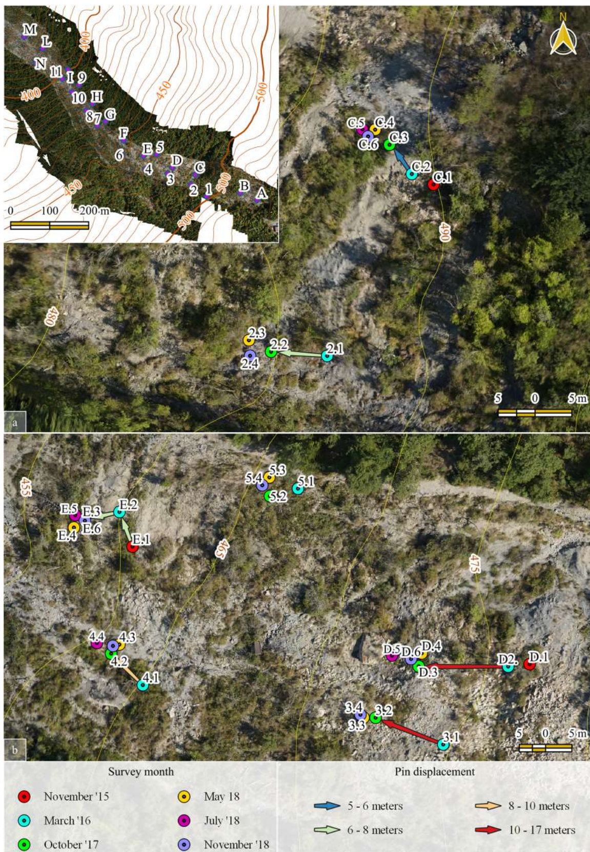
Fig. 5 Pins with the largest displacements in the observed period. (a) Detachment niche zone near Casale S. Antonio. (b) Highest displacement zone, located downvalley of the landslide terrace.
