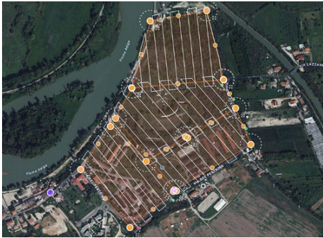
Fig. 8- Photogrammetric acquisition schema of the whole area
