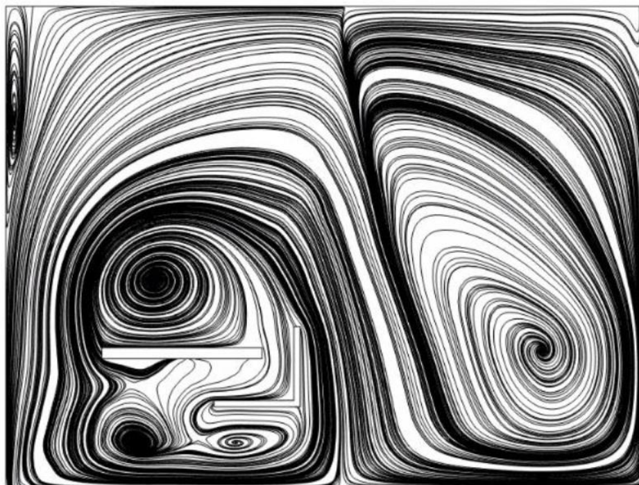
Figure 37. Streamlines behaviour in presence of obstacles, yz plane, Cut Plane at x = 0.7
