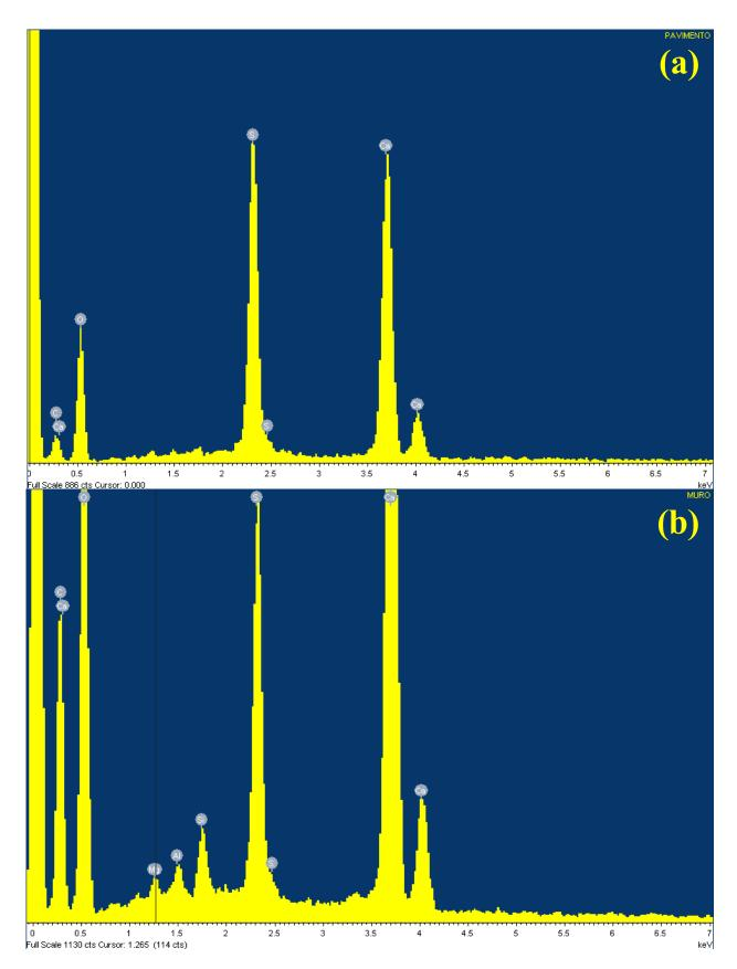
**Figure 5.** EDS spectra of (**a**) floor sample and (**b**) wall sample. For experimental condition: see Section 4 (Materials and Methods).
