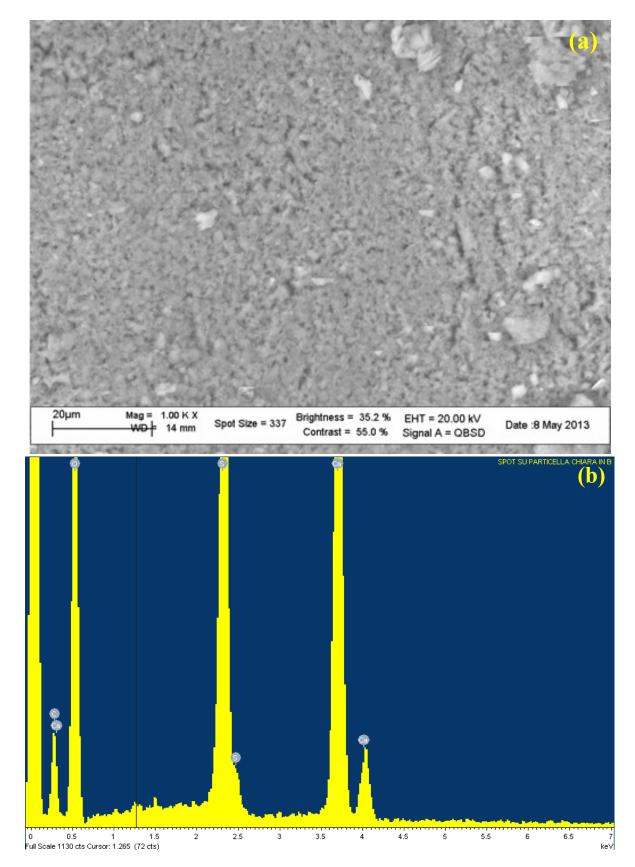
**Figure 6.** SEM photo (**a**) and EDS spectrum (**b**) of the spot of the particle "A" of the wall sample. For experimental condition: see Section 4 (Materials and Methods).
