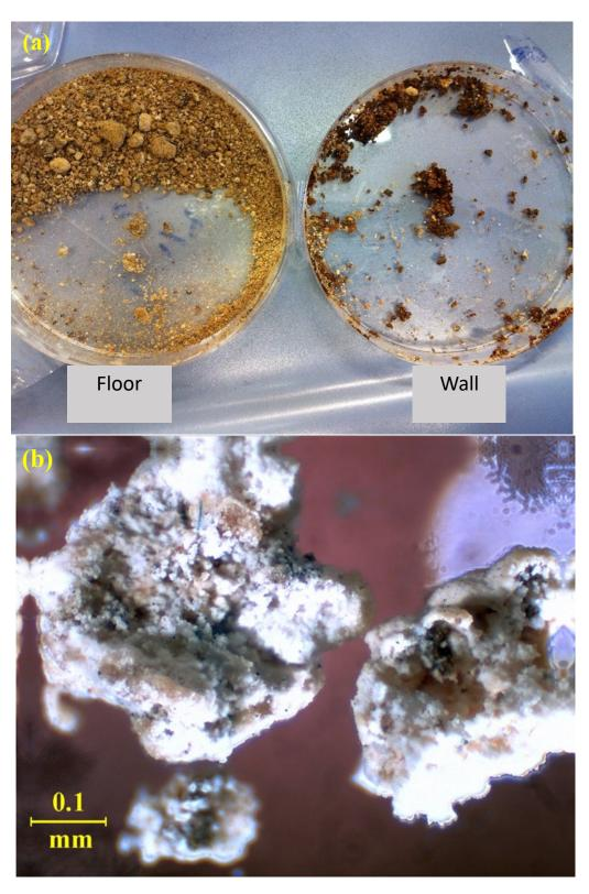
**Figure 3.** (a) Photo of the samples of the degradation product of both the floor and the wall (glass Petri plate 80 mm); (b) photo of the degradation product of the pavimental mosaic taken by the optical microscope (1000× magnification; width focusing 25 mm, 2 mm increments; 6 V/20 W halogen light).
