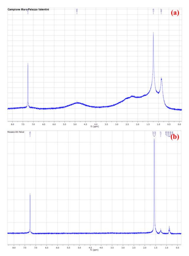
**Figure 7.** <sup>1</sup>H-NMR spectra (300 MHz, CDCl<sub>3</sub>) of (**a**) wall and (**b**) pavement samples.
