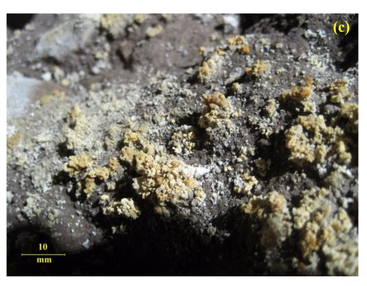
**Figure 2.** Photos of the degradation (**a**) of the floor and (**b**) of the wall and optical microscope image (**c**) on the surface of the black and white mosaic pavement ( $10 \times$  and  $40 \times$  magnification, respectively; width focusing 25 mm, 2 mm increments; 6 V/20 W halogen light). The sample of the degradation product of the black and white pavement mosaic of *domus B* was analyzed under an optical microscope in transmittance and reflectance).
