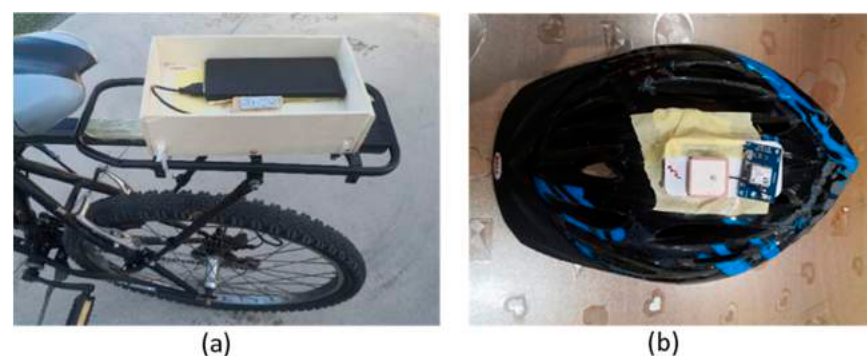
Figure 14. Installation of the prototypes on the bike: (a) Bike-frame and (b) Bike-helmet details.
