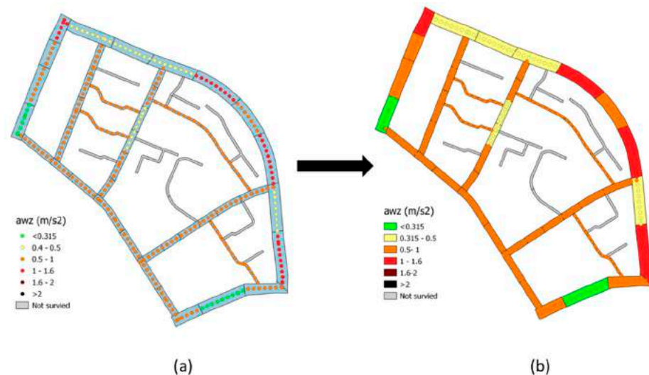
Figure 9. Visualization of a_{wz} results in GIS: (a) point representation (b) sample unit representation.
