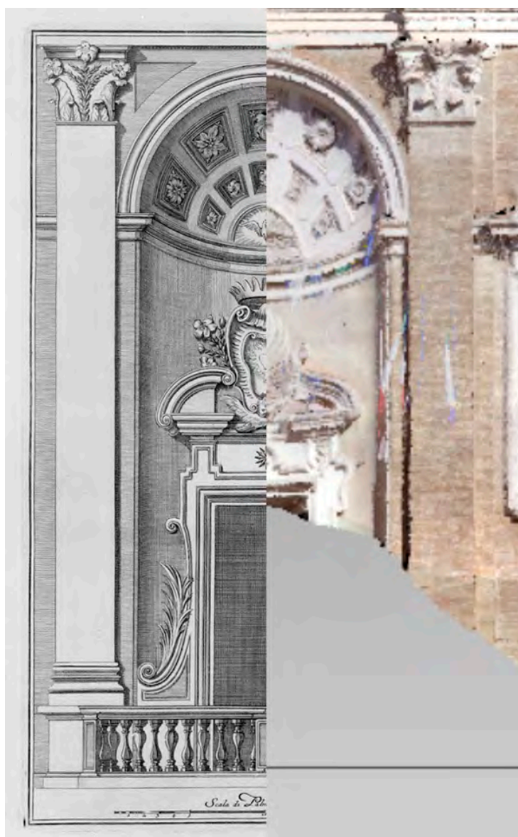
Figure 15. Comparison between Sebastiano Giannini's plate of the portal in the niche and the orthographic elevation after the photographic model (elaboration of the authors).
