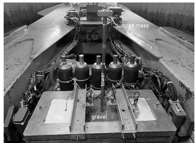
Fig. 2. Model loaded on the centrifuge.
