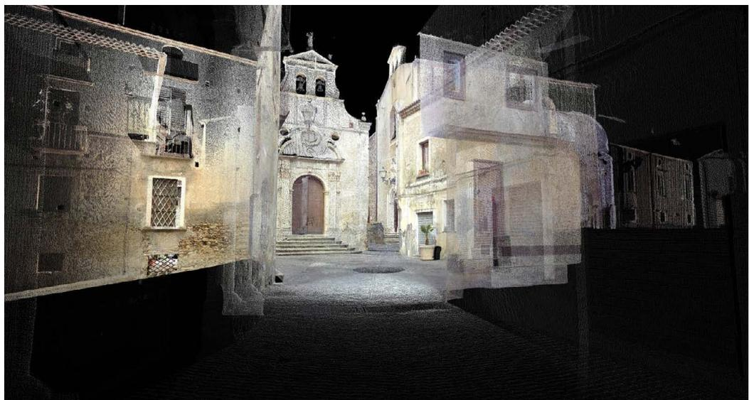
Fig. 6. The Church of the Addolorata, numerical model derived from laser scan processing. Elaboration of the authors.
