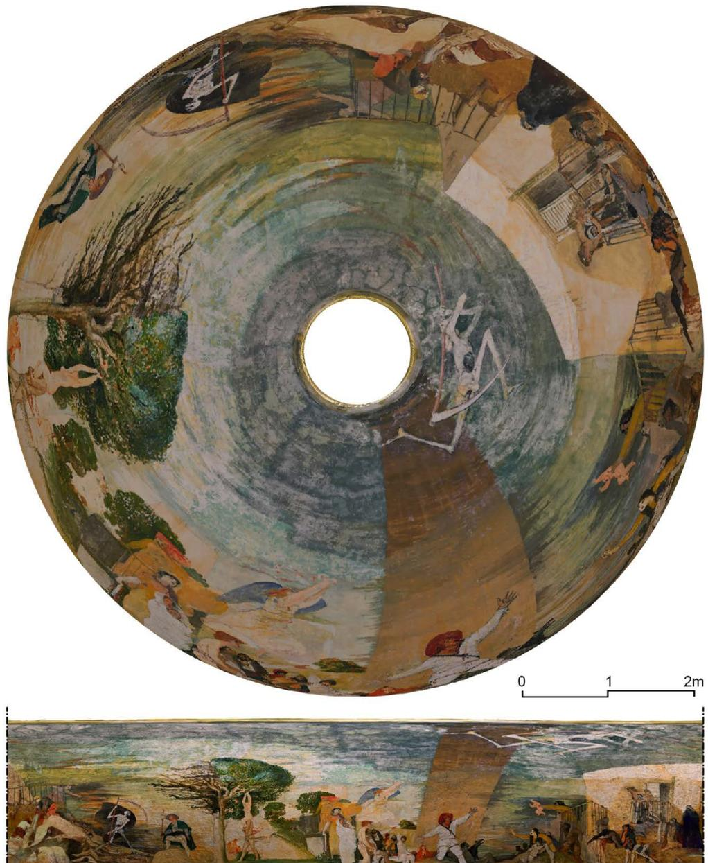
Fig. 11. The dome of the Church of San Rocco. At the top, the orthophoto, at the bottom the development of the painted surface. Elaboration of the authors.
