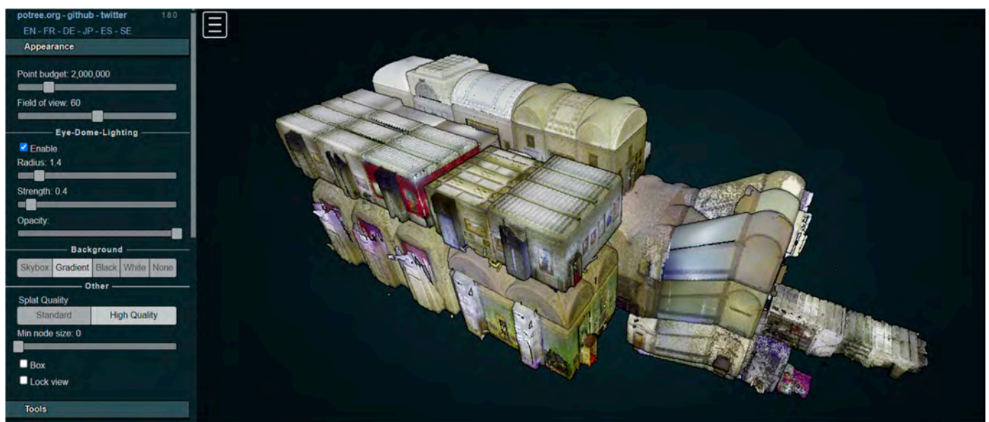
Figure 7. Point cloud of the test area uploaded to a local server and visualized in Potree viewer.
