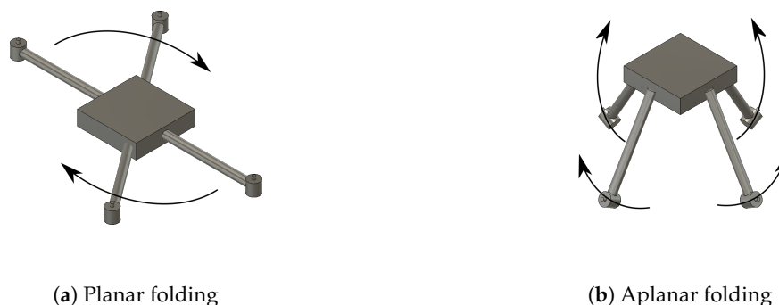
Figure 8. Reconfigurable folding options.
