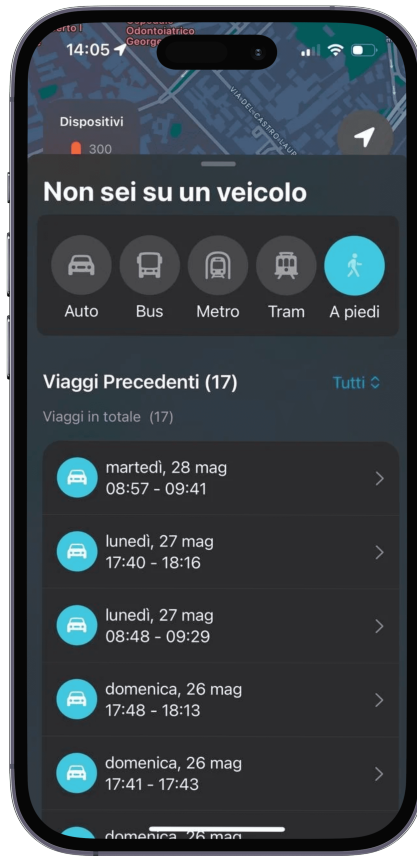
Figure 3.1. Trip history interface showing mode classification, timestamps, and quick visual summaries. Translation: "Non sei su un veicolo" = "You are not in a vehicle", "Auto" = "Car", "Bus" = "Bus", "Metro" = "Subway", "Tram" = "Tram", "A piedi" = "On foot", "Viaggi Precedenti" = "Previous trips", "Tutti" = "All". Dates and times (e.g., "martedì, 28 mag" ) indicate the day (Tuesday, 28 May).
