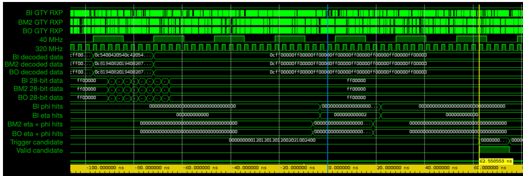
Figure 7.8. Snapshot of the SL firmware simulation showing the GTY RX signals, the 40 MHz and 320 MHz clocks, the decoded data, the 28-bit DCT data, the hit frames and the valid trigger candidate. The blue cursor indicates the time the hit frames are received by the trigger logic, while the yellow cursor the time a trigger candidate is generated.
