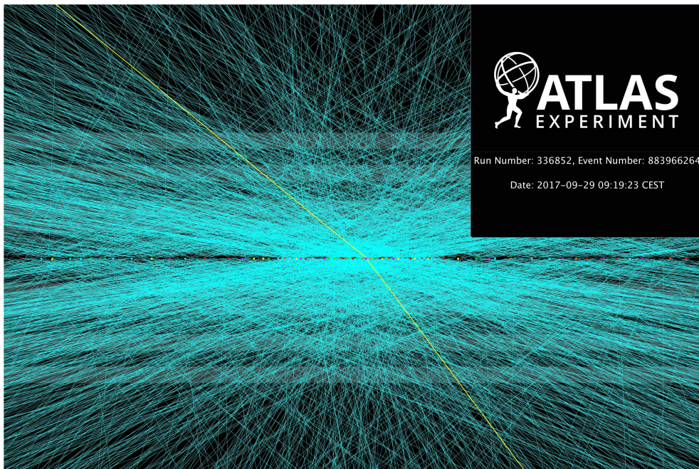
Figure 3.1. Event display for a Z \rightarrow \mu\mu candidate event with 65 additional reconstructed primary vertices recorded by ATLAS in 2017 [64].
