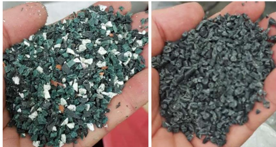
Figure 1. Comparison of polyolefins before (left) and after (right) homogenization treatment.
