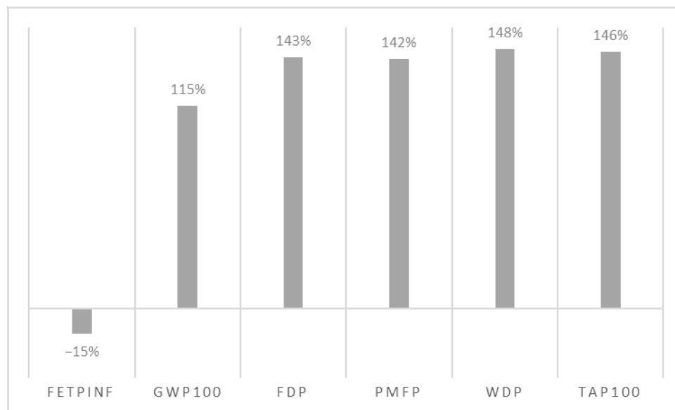
Figure 14. Percentage variation in each impact category for the recycled plastic scenario compared to the virgin plastic scenario. FETPINF: freshwater ecotoxicity; GWP100: climate change; FDP: fossil depletion; PMFP: particulate matter formation; WDP: water depletion; TAP100: terrestrial acidification.
