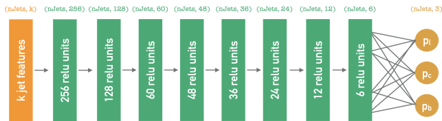
Figure 3.11. Schematic drawing of the DL1r neural network architecture. A similar architecture is used for DL1d from Ref. [73].
