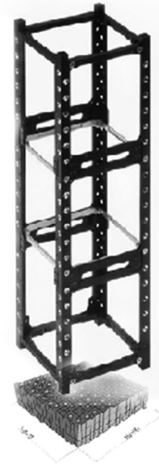
Fig. 18. Schematic view of the microrockets assembly.
