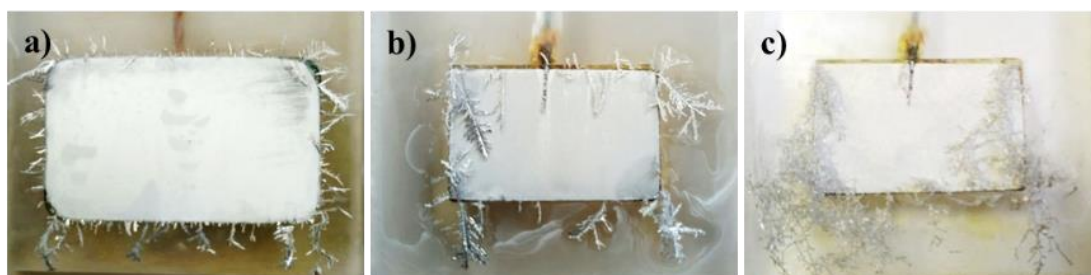
Figure 19. Dendritic growth as CD increases from 100 to 300 A/m 2 using a sulfate electrolyte and the AISI 316L cathode.
