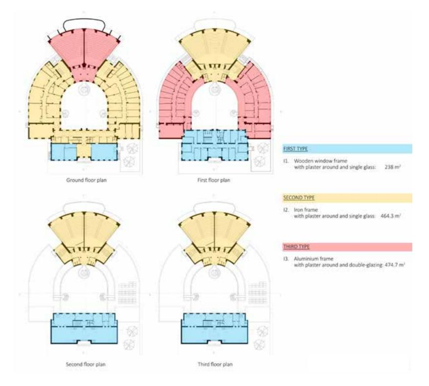
Figure 29 - Mapping of types of window frames in wood, iron and aluminum (© Romano 2020)
