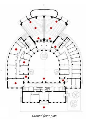
Figure 34 - Positioning of measuring points for IAQ sampling at the three levels of the building (© Mancini, Romano 2020)
