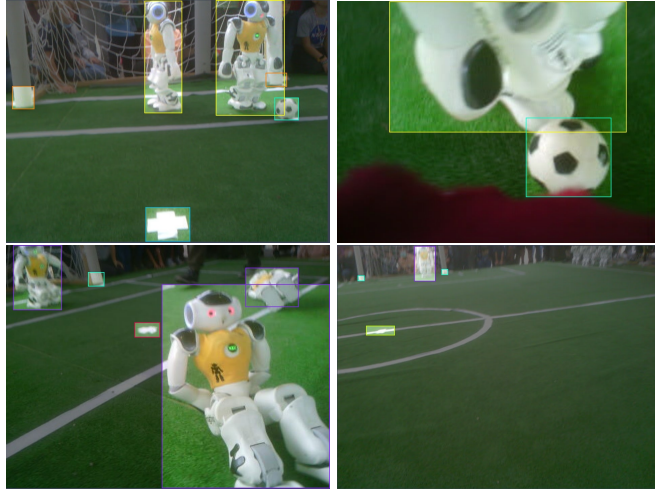
Fig. 2: Examples of labeled images taken from SPQR Dataset. The images also include samples with natural light conditions and noisy backgrounds, which make the detection more challenging for lightweight neural networks.
