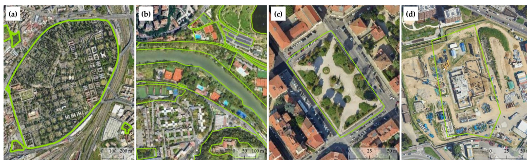
Figure 5. Examples of some types of areas mapped by UA as “1.4—Artificial non-agricultural vegetated areas” excluded from the accessibility assessment thanks to the filter on the maximum percentage of consumed land, such as cemeteries (a), sports fields (b), highly artificialized squares (c), and areas affected by land consumption (d).
