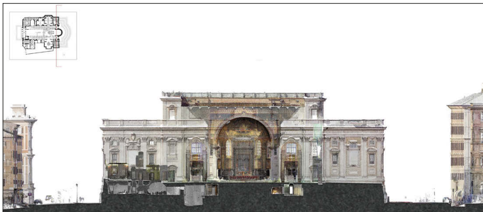
Fig. 4 – Cross section-laser scanner point cloud.
