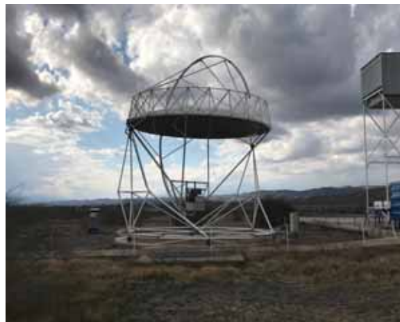
Figure 6. Dish/Engine system (credits © H2020 European Nexttower Project).
