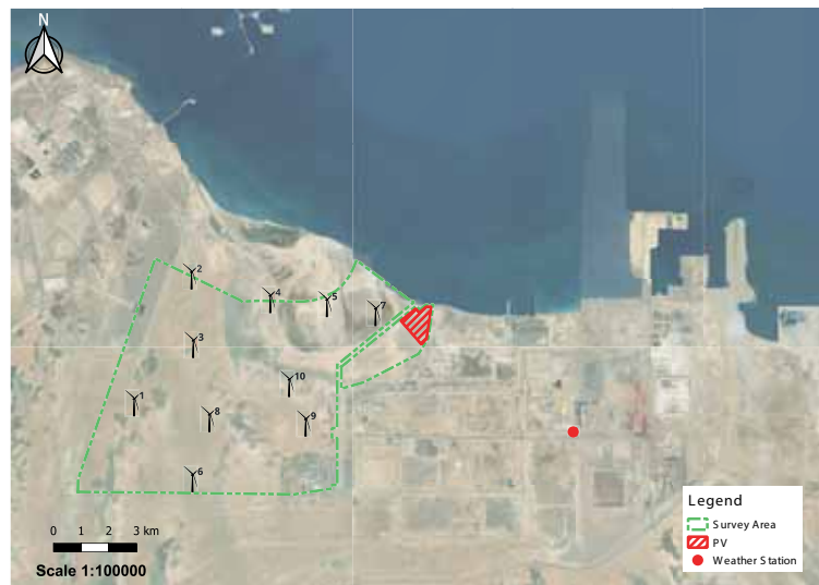
Figure 14. Arrangement of 10 wind turbines (corresponding to the turbines listed in Table 6) and land-based PV modules for the proposed hybrid farm.
