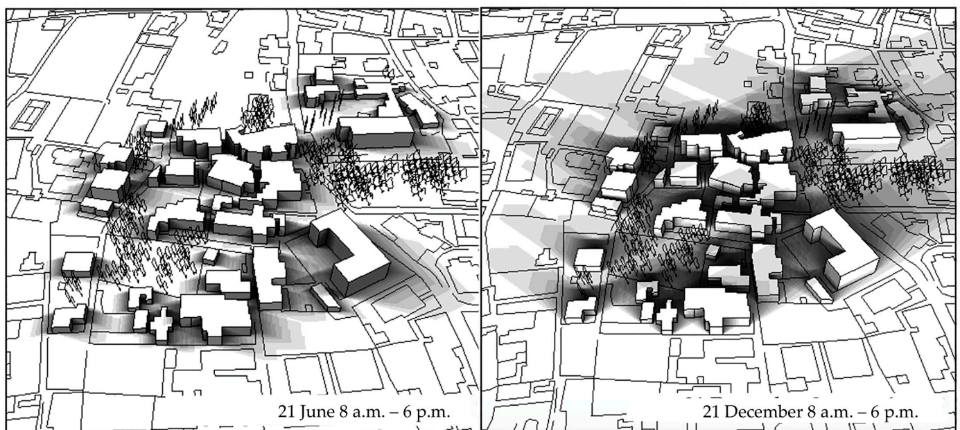
Figure 13. (left) Shading of the area on 21 June; (right) shading of the area on 21 December.
