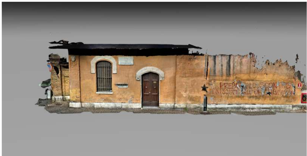
Fig. 12. Rendering of a work portion of the 3D model with textures obtained from the processing of data acquired with the iPad with the Polycam software and rendered with the Rhinoceros 7 software (elaboration of the authors).
