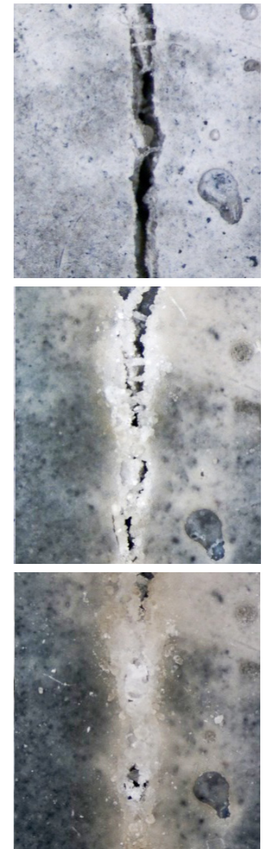
22. Bioconcrete, self-healing concrete, Henk Jonkers
