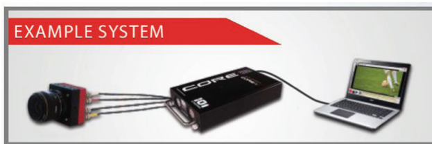
Fig. 2. Image-based acquisition system: high-speed camera, core and PC.
