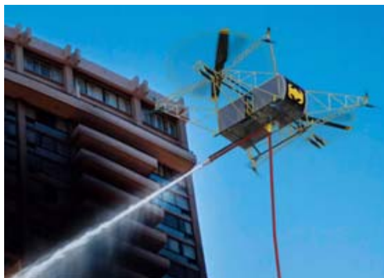
Figure 7. Drone connected with a pipe used for firefighting on a building
