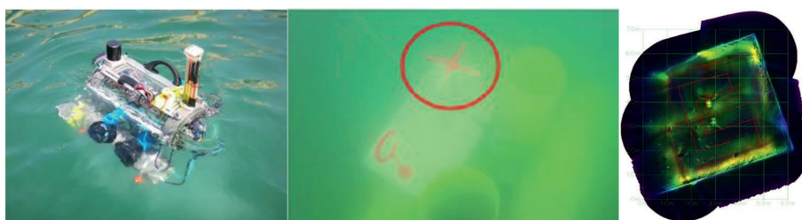
Figure 5. (left) the Feelhippo AUV from the UNIFI robotics team in action. (Centre) the yellow pipe structure with the manipulation console used in the ERL emergency competitions. (right) a multi-beam mosaic by team Tomkyle of the competition area. The different objects of potential interest (buoys, pipeline assembly structures, the gate are visible).
