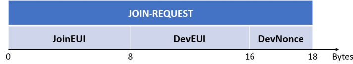
Figure 3.4. Join request message structure.
