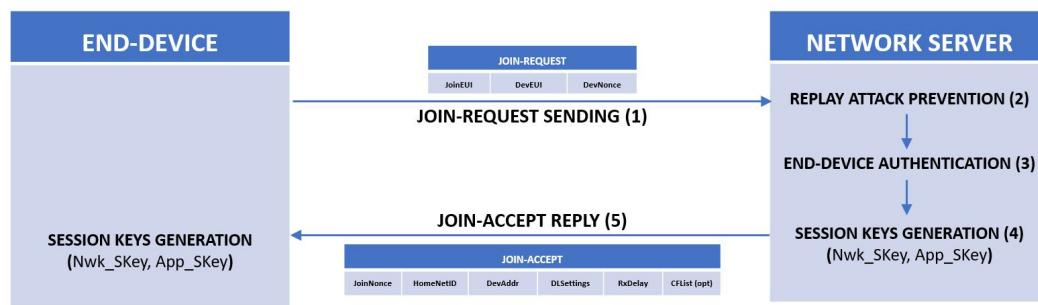
Figure 3.3. Over-The-Air Activation (OTAA) procedure flow graph.
