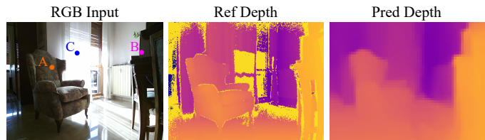
Fig. 7: METER application in a real-case scenario. Missing depth measurements of reference (Ref) depth are shown as yellow pixels. A uniform colormap, with the same depth range, has been applied to the depth maps. Points A (armchair), B (box), and C (curtain) on the RGB frame indicates object used for quantitative comparison.
