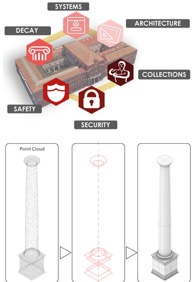
Fig. 1 - HBIM involves several actors of various cognitive domains ranging from history, restoration, technology, diagnostics, etc., whose work produces information to be included and shared within the model.
