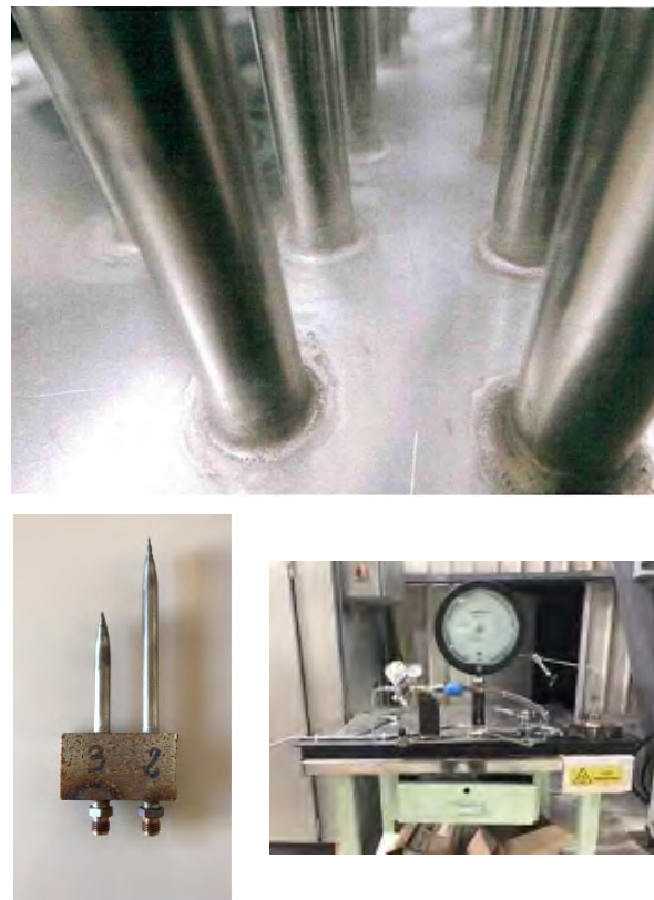
Figure 2. Examination and testing of the joining solution. From the top: detail of the stereoscope analysis; picture of two pressure test samples; pressure test device.
