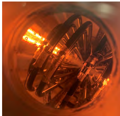
Figure 12. Picture of the niobium pipes heated by the infrared lamps from the viewport installed on the top of the PAV-ONE vessel.
