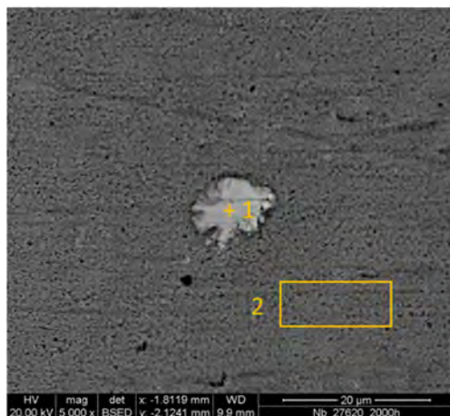
Figure 9. Longitudinal SEM image and elemental composition via EDX of uncleaned Nb sample after 2000 h.
