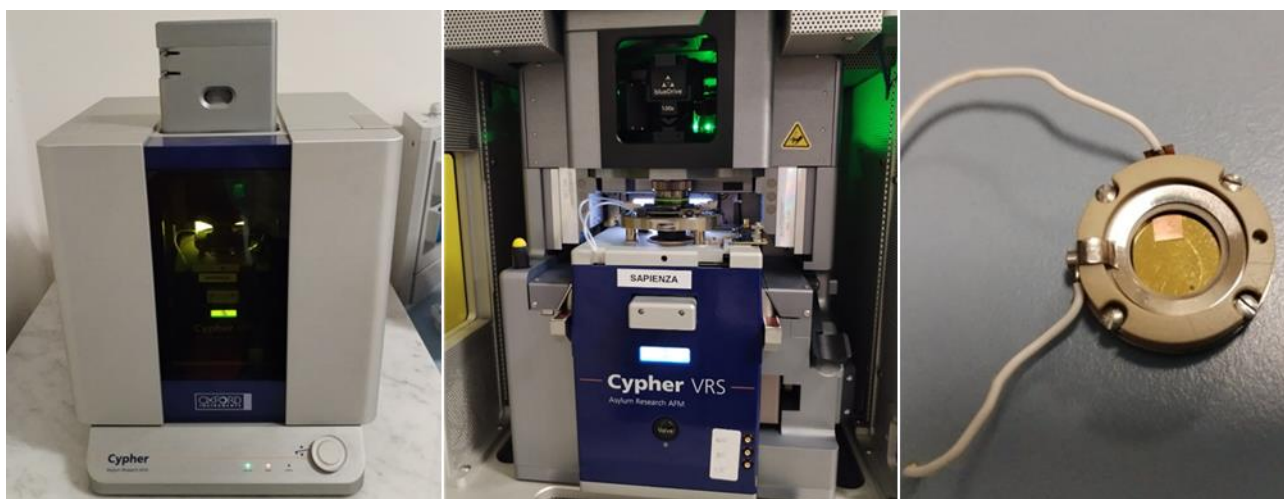
Figure 5-3 AFM Cypher VRS instrument and electrochemical cell for integrated EC-AFM
