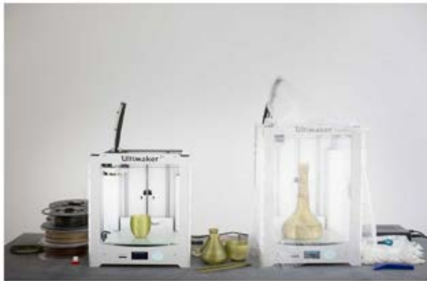
Figure 4. 3D printing of vases created with a biopolymer derived from algae to replace the use of plastic. The production is located within the Algae Lab bio-laboratory of Atelier LUMA and Studio Klarenbeek & Dros, which focuses on studying local renewable resources to propose circular and decentralized production.
