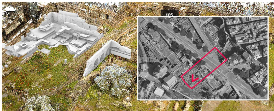
Overlay of the informed model developed using VPL and the point cloud of a portion of the Forum of Nerva.
