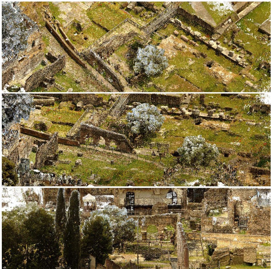
Fig. 7. Views of the point cloud generated by acquisition through 3D Laser Scanner:
