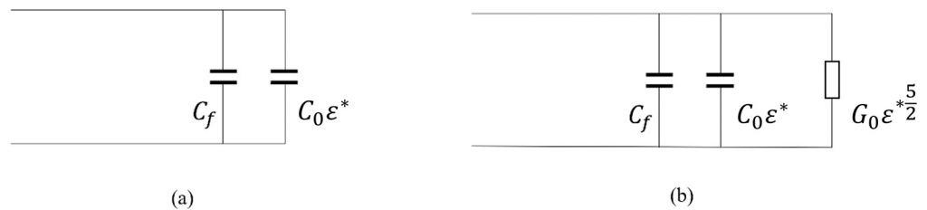
Figure 3. (a) Equivalent circuit of the S&S de-embedding model; (b) Equivalent circuit of the M&E de-embedding model.
