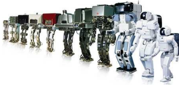
Figure 2.4. Honda E series (E0 in 1986 to E6 in 1993) robots, Honda P series (P1 in 1993 to P3 in 1997) robots, and ASIMO (2000) [4].
