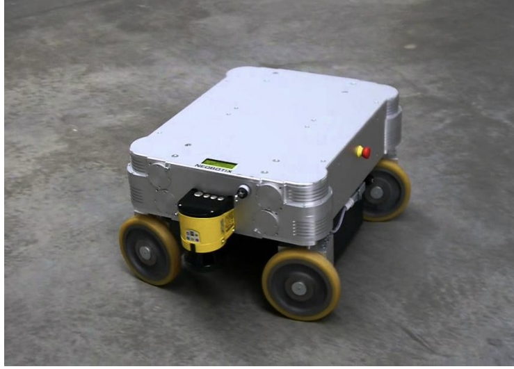
Figure 9.1. The Neobotix MPO-700 steerable wheeled mobile robot.
