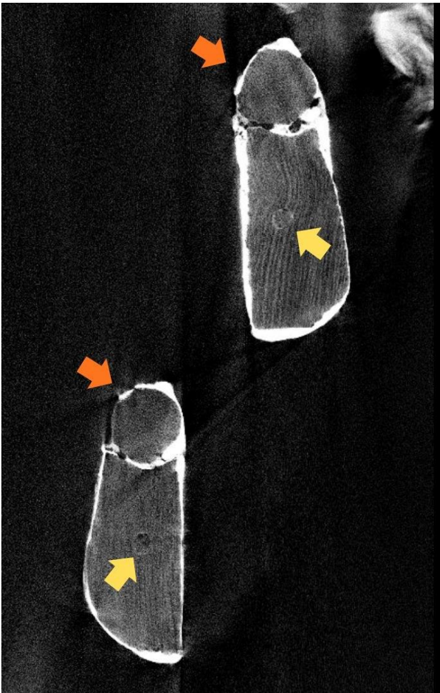
Fig. 51 – Bearer C, transversal slice of the feet. Orange arrows: lower portion of the legs. Yellow arrows: dowel inserted on the centre of the feet
