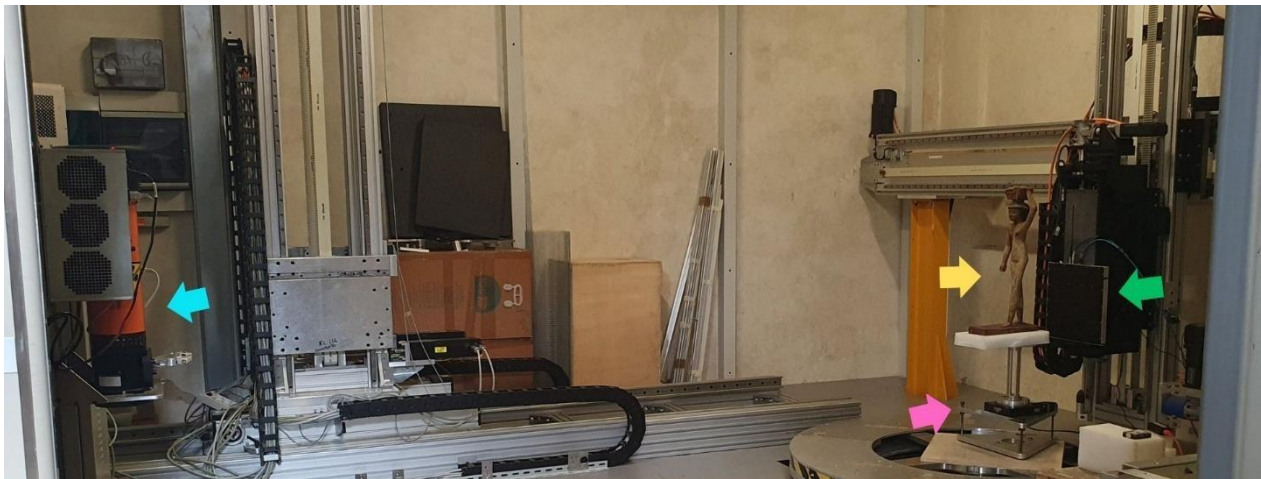
Fig. 11 – CT setup, Bearer 8794 (Bearer C). Light blue arrow: source; Pink arrow: rotating platform; Yellow arrow: Bearer C; Green arrow: detector
