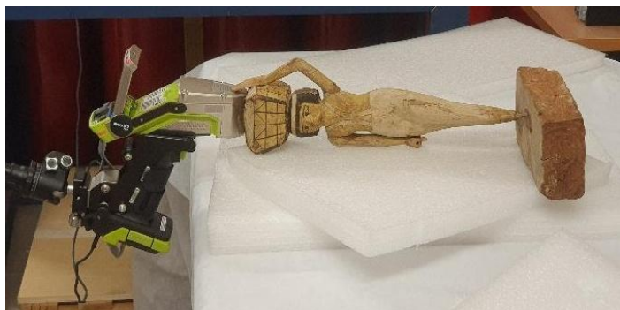
Fig. 14 – THERMO Niton XL5 Plus portable spectrometer, measurement on Bearer B
