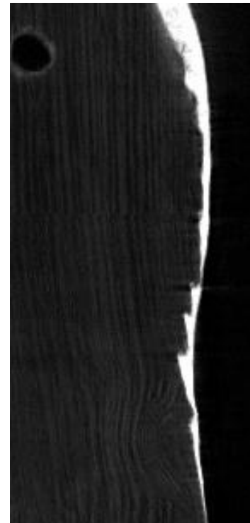
Fig. 36 – Bearer A, back area discontinuities attributable to tool marks
