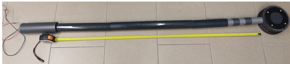
Figure 1. The prototype of the FlashDC experiment, unmounted from the linac BEW.
