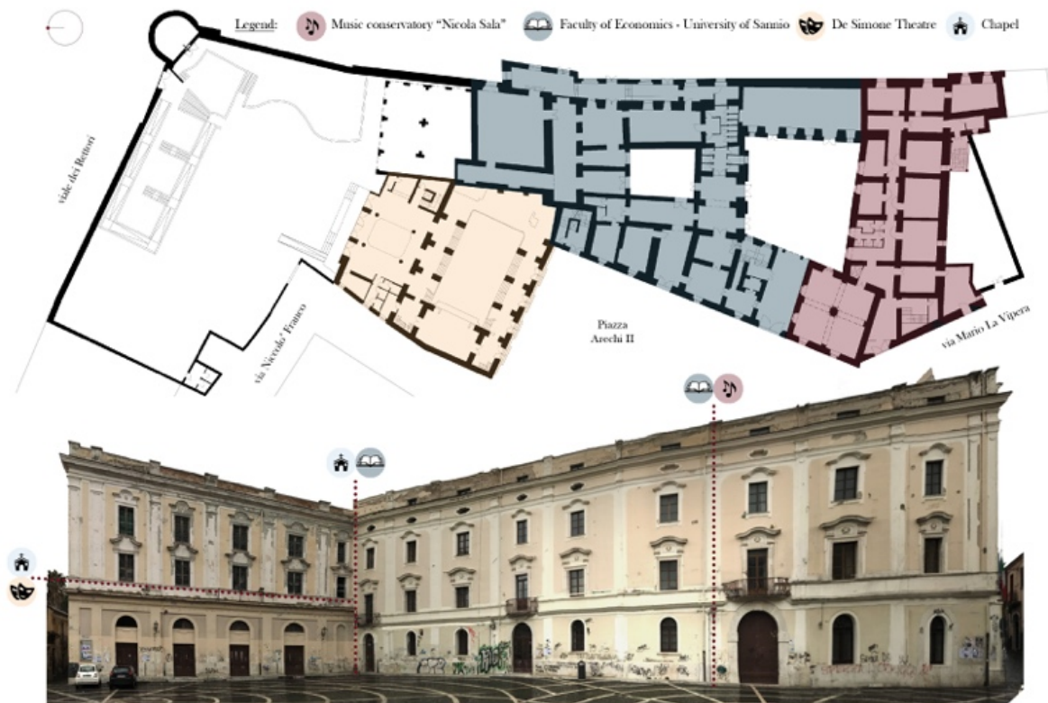
Figure 2. Ground floor plan and main façade of Palazzo De Simone straightened from a photo taken from Piazza Arechi II in its current condition.
